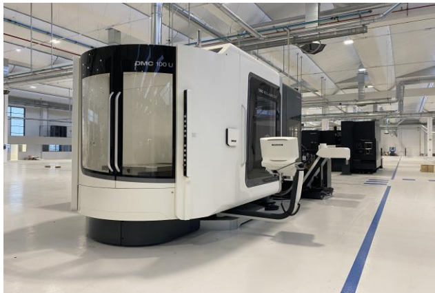
New Machining Centre DMC 100U duoBLOCK for the processing of EFP-1 Engine Flywheel PTO
